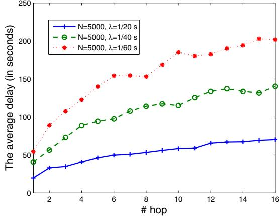
Fig. 7. The average delay varies with the number of hops, under  $N = 5000$  and different  $\lambda = 1/20$  s,  $1/40$  s,  $1/60$  s
